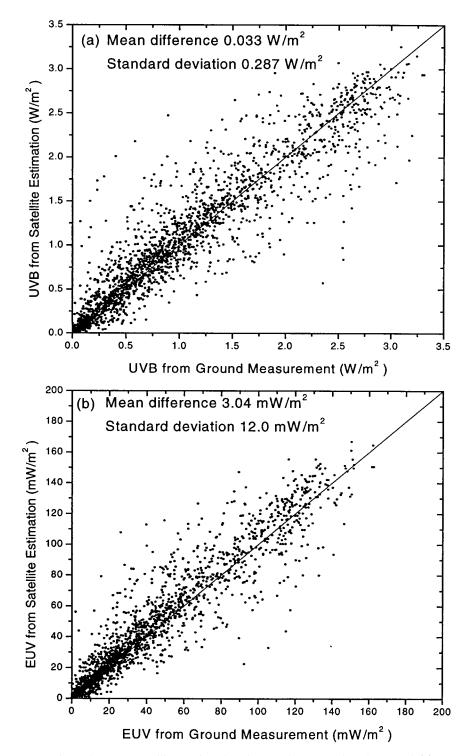
**Figure 2.** Comparisons between satellite-retrieved and ground-measured surface total (a) UV-B and erythemal (b) UV under all-sky conditions from 1992 to 1994. Satellite estimation was made using TOMS data, while surface data are from Canadian UV stations.
