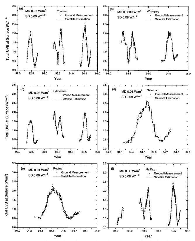
**Figure 4.** Comparisons of 10-day running mean surface total UV-B between satellite estimation and ground measurement at all Canadian UV stations. Mean and standard differences (MD and s.d.) are also given.
