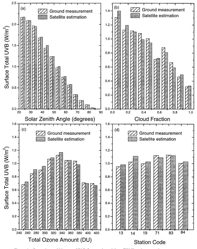
Figure 6. Comparisons of bin mean UV-B fluxes estimated from TOMS against ground measurements (1992–1994) averaged over various intervals in (a) solar zenith angle (b), cloud fraction (c), total ozone amount, and (d) stations.
