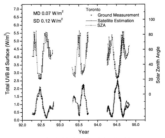
Figure 5. Comparison of variations in UV-B flux and solar zenith angle for Toronto.
