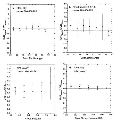
**Figure 7.** Ratios of estimated and observed surface UV-B fluxes averaged in the bins sorted with restrictions as specified in the plots by (a, b) solar zenith angle, (c) cloud fraction, and (d) ozone amount. Figures 7a and 7b are mostly clear and cloudy conditions, respectively.
