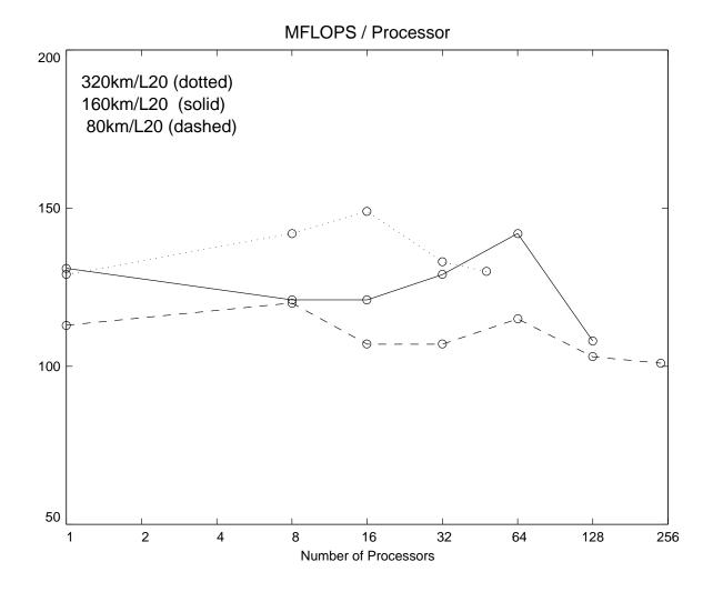
FIGURE 6. MFLOPS per processor achieved by SEAM at three different model resolutions and up to 240 processors.
