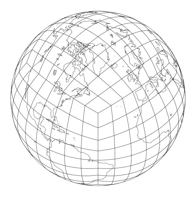
FIGURE 1. The cube projected onto the sphere. Each of the 6 faces of the cube has been divided into an  $8 \times 8$  array of elements. Within each element we would typically use an  $8 \times 8$  Gaussian grid and 20 vertical levels. This results in approximately 160 km horizontal resolution.
