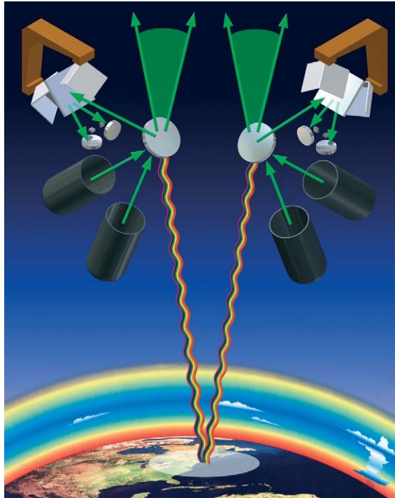
Fig. 1. Instrument configuration. A key design feature is the use of dual FTSs bore-sighted on the same nadir footprint. Each instrument is a four-port, cube-corner FTS, each with two blackbodies that overdetermine the calibration, and with a deep space view over 45^\circ to calibrate polarization errors.
