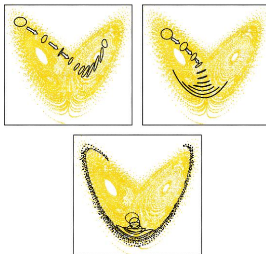
Figure 1: The scientific basis for ensemble prediction illustrated by the prototypical Lorenz model of low-order chaos, showing that in a nonlinear system, predictability is flow dependent. (a) A forecast with high probability, (b) forecast with moderate predictability, (c) forecast with low predictability.
