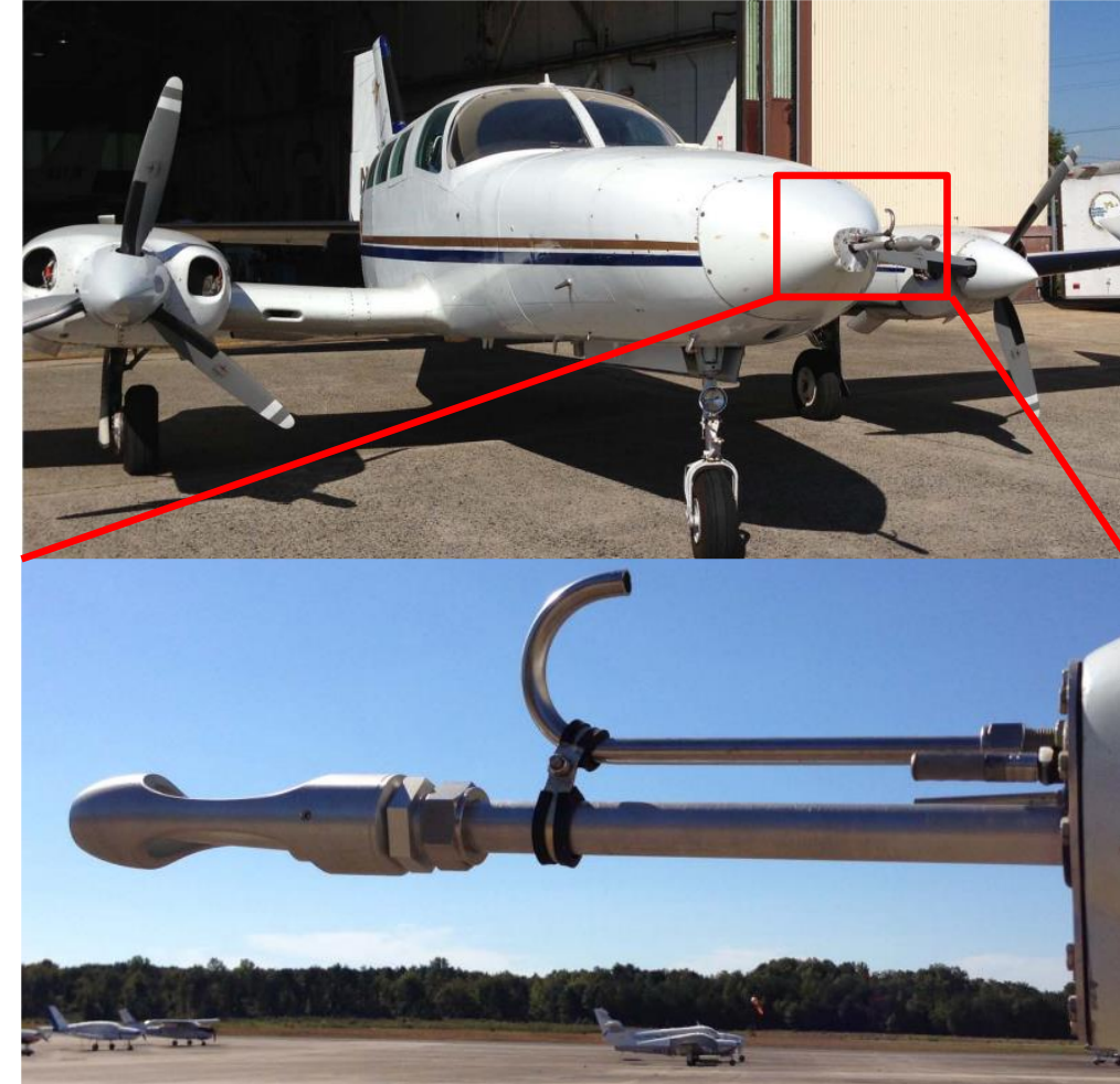
Figure 1 (top): UMD Research Cessna 402B with a red box highlighting the (bottom) "candy cane" inlet, Aerosol inlet and met (T/RH) sensors
