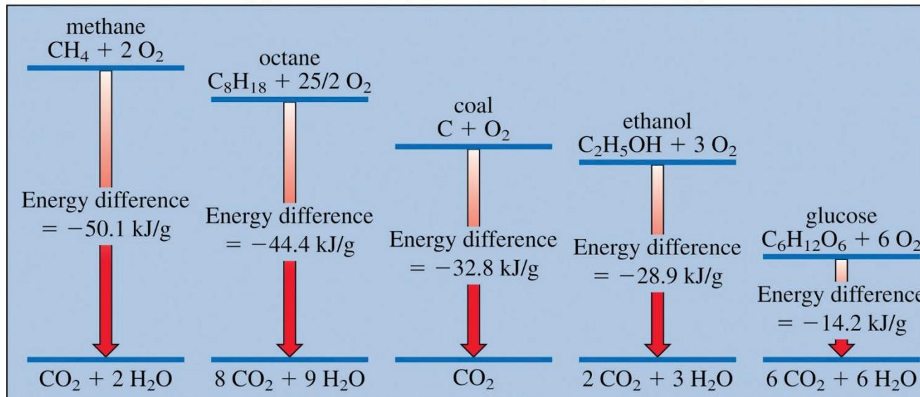
Fig 4.26. Energy differences (in kJ/g) for the combustion of methane ( $\text{CH}_4$ ), n-octane ( $\text{C}_8\text{H}_{18}$ ), coal (assumed to be pure carbon), ethanol ( $\text{C}_2\text{H}_5\text{OH}$ ), and wood (assumed to be glucose).
