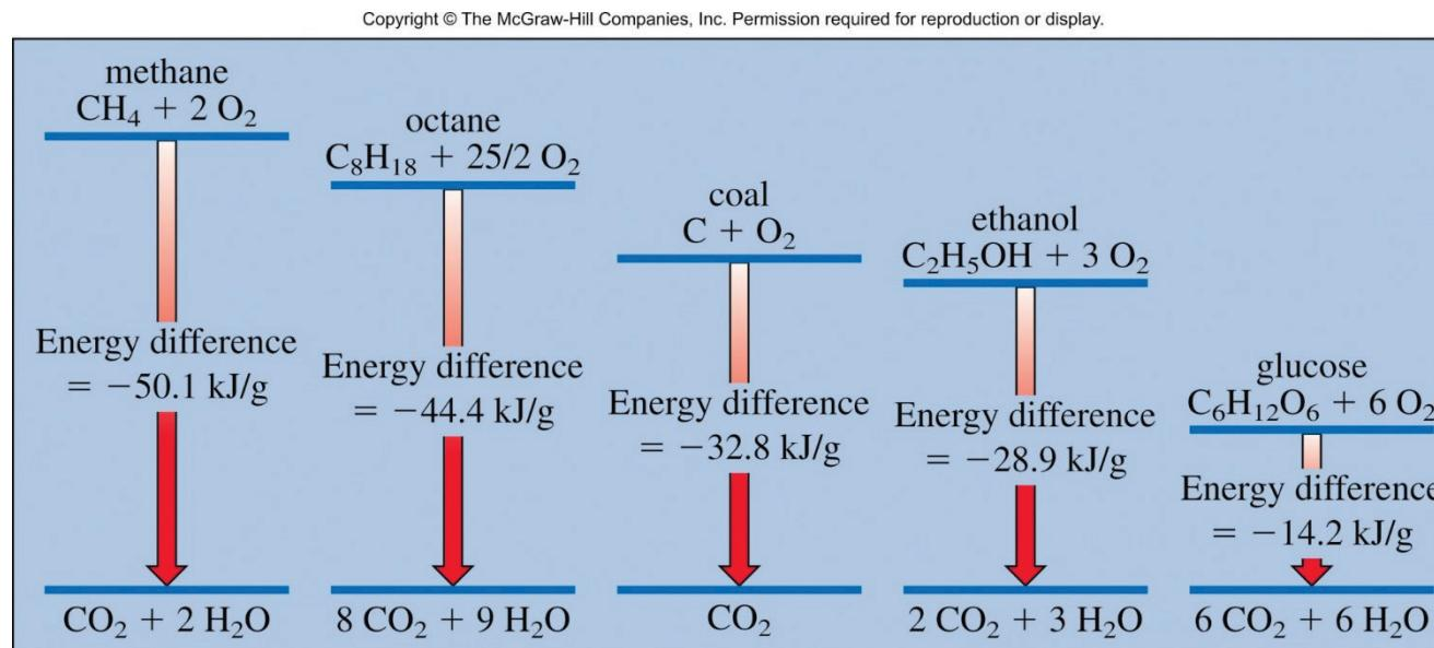
Fig 4.26. Energy differences (in kJ/g) for the combustion of methane ( $\text{CH}_4$ ), n-octane ( $\text{C}_8\text{H}_{18}$ ), coal (assumed to be pure carbon), ethanol ( $\text{C}_2\text{H}_5\text{OH}$ ), and wood (assumed to be glucose).
