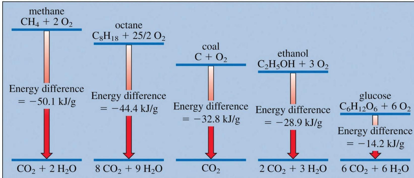
Fig 4.16. Energy differences (in kJ/g) for the combustion of methane ( $\text{CH}_4$ ), n-octane ( $\text{C}_8\text{H}_{18}$ ), coal (assumed to be pure carbon), ethanol ( $\text{C}_2\text{H}_5\text{OH}$ ), and wood (assumed to be glucose).
