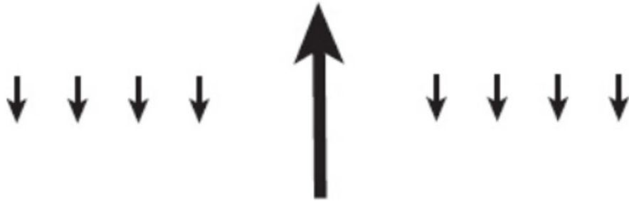
Figure 3.6. Sketch illustrating a strong updraft, represented by the large arrow, and surrounding weak downdrafts, represented by the small arrows. The upward and downward mass flows can cancel.
