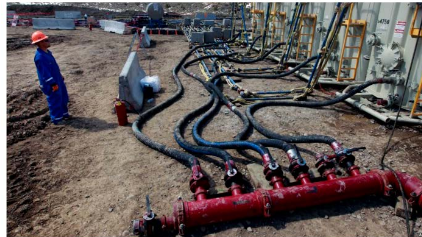
A worker helps monitor water pumping pressure and temperature, at a hydraulic fracturing and extraction site, outside Rifle, in western Colorado, March 29, 2013.
