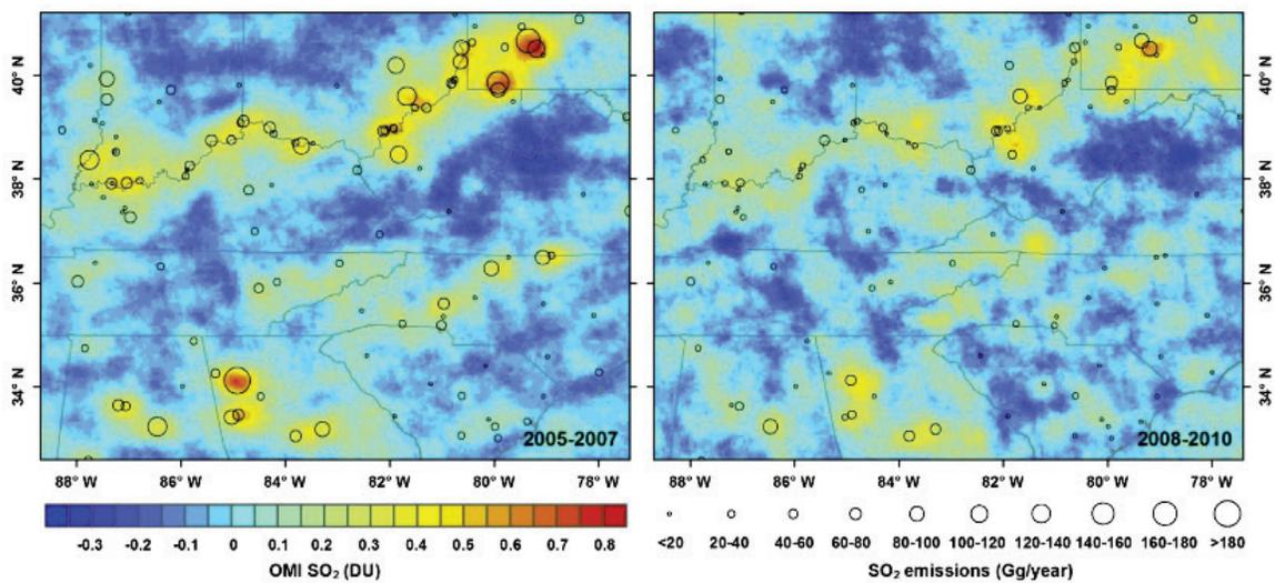
Fig. 4. Mean SO<sub>2</sub> burdens over the Ohio River Basin for 2005–2007 (left) and 2008–2010 (right) measured by OMI, confirming a substantial reduction in SO<sub>2</sub> pollution around the largest coal-fired power plants, as a result of the implementation of SO<sub>2</sub> emission control measures (adapted from NASA Earth Observatory, as reported in Fioletov et al., 2011).
