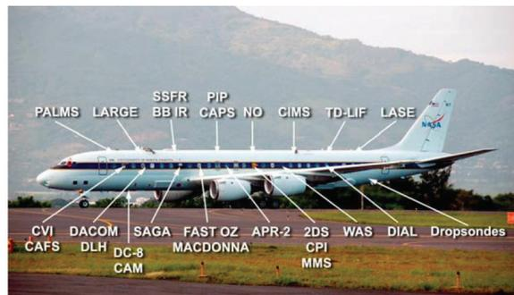
**Figure 5.** The NASA DC-8 showing the instruments used in TC4 and their placement on the aircraft.
