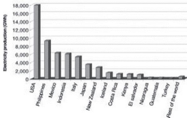
Figure 8.5 Geothermal electricity production, 2005. (Source: Bertani, R. [103].)
