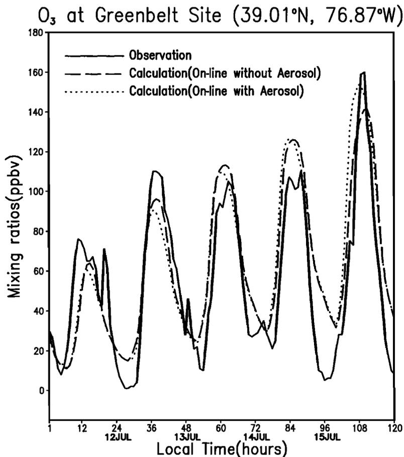
**Figure 3.** Time series of surface  $O_3$  at Greenbelt site. Solid line is  $O_3$  observed, dotted line is  $O_3$  calculated with diurnally varying aerosols in the boundary layer, and dashed line is  $O_3$  calculated without aerosols.
