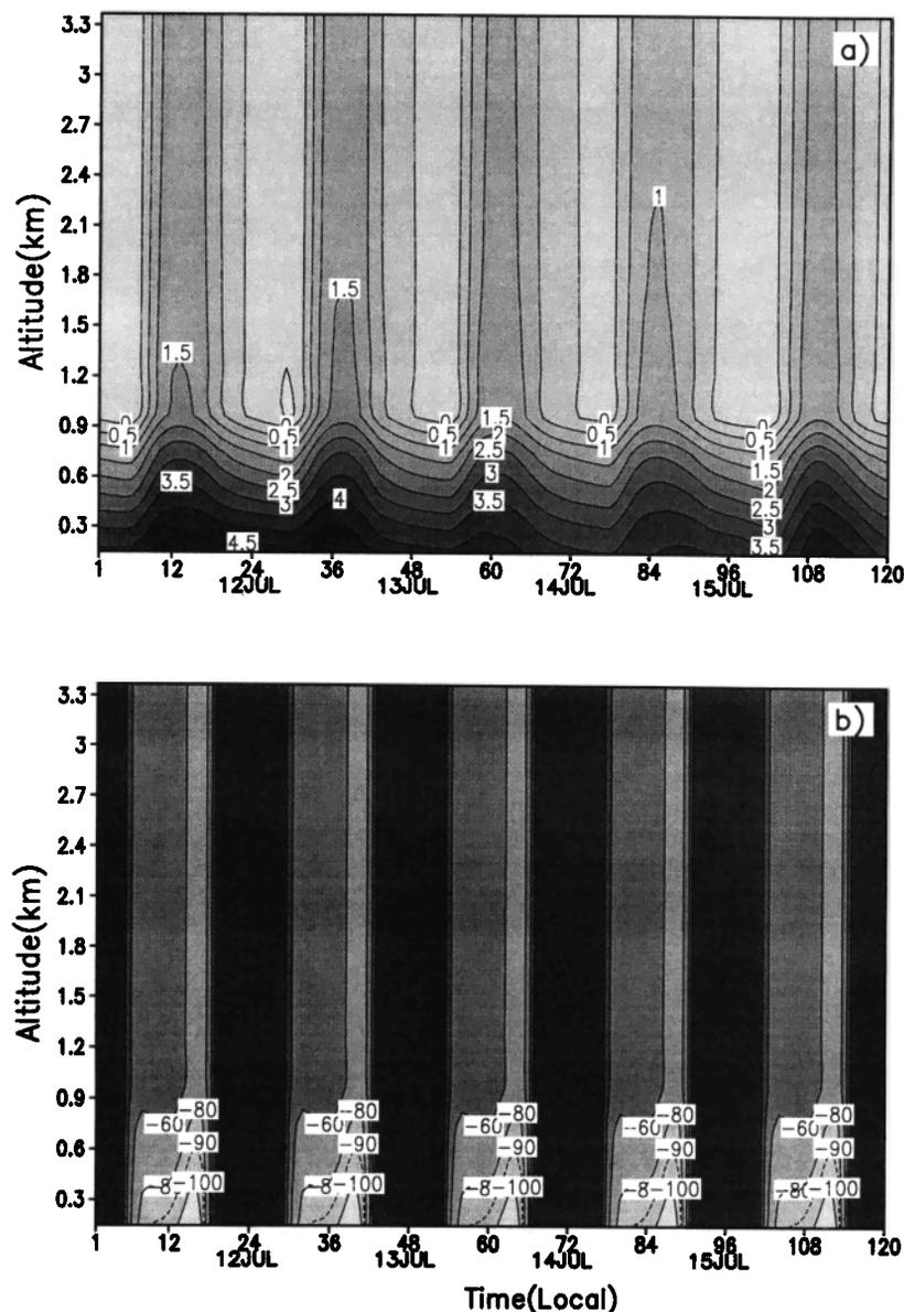
**Figure 6.** Radiative forcing due to the presence of aerosols for July 11–15, 1995, at Greenbelt, Maryland. (a) Changes in net longwave fluxes (downward) and (b) changes in net shortwave fluxes (downward) with aerosols versus with no aerosols ( $\text{W m}^{-2}$ ).
