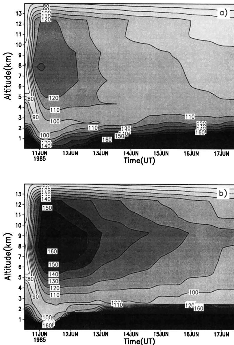
**Figure 7.** CO tracer analysis simulated with single-column chemical transport model (SCCTM) for (a) rural air and (b) urban plume vertically redistributed in June 10–11, 1985, Kansas/Oklahoma PRESTORM convective event.
