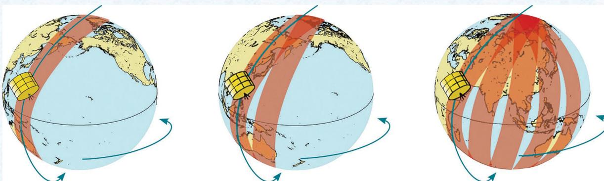
**Polar orbiting satellites:** Travel over the poles. Orbits wrap around the Earth. Need to travel quickly to provide cover the globe. Can be very high resolution because they orbit closer to the surface than geostationary satellites
