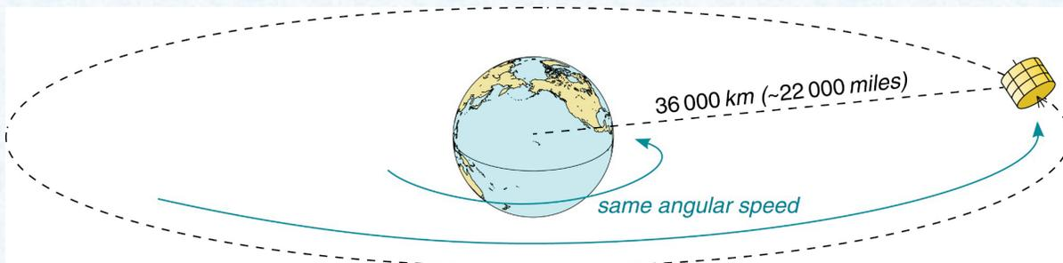
**Geostationary satellites:** Orbits the Earth at the same angular speed as the Earth. They are “parked” in orbit over Earth and stay over the same location.
