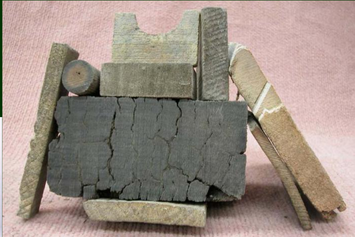
Wood in a landfill after 46 years, Australia Ximenes et al., 2008
