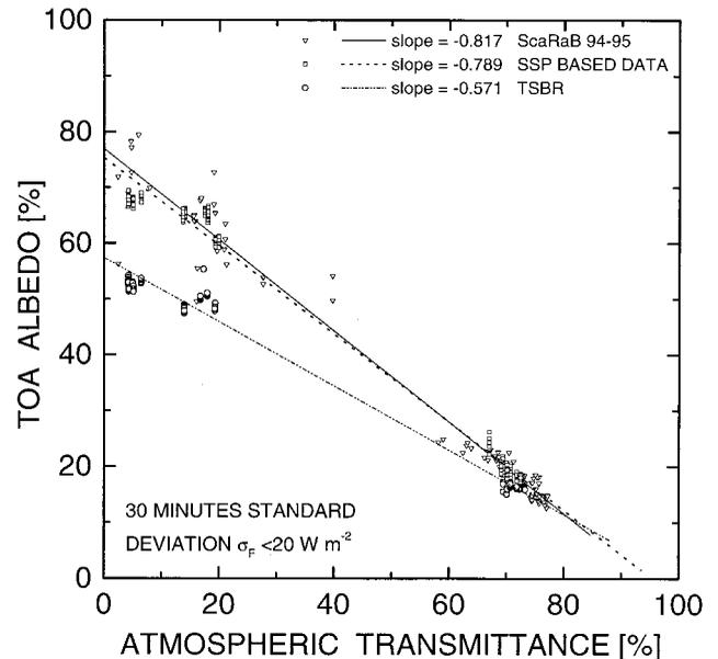
**Figure 7.** The relationship between top of the atmosphere (TOA) albedo and atmospheric transmittance. TOA albedos were derived from ScaRaB, SSP, and TSBR. Atmospheric transmittances were computed from Baseline Surface Radiation Network (BSRN) surface irradiance measurements. Slopes of the linear egressions are listed on the plot.
