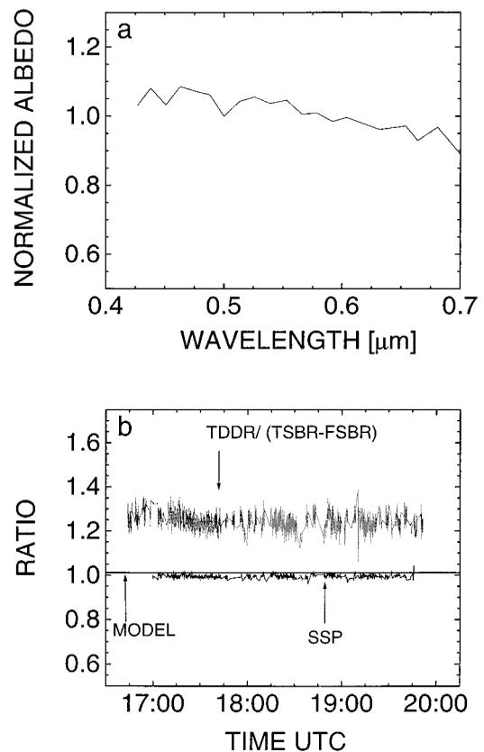
**Figure 4.** (a) An averaged sample of spectral variation of monochromatic albedo observed by SSP on October 30, 1995, normalized to albedo value at 500 nm. (b) The ratio of albedos at 500 nm and in the visible region obtained from SSP, a combination of TDDR, FSBR, and TSBR, as well from model calculation.
