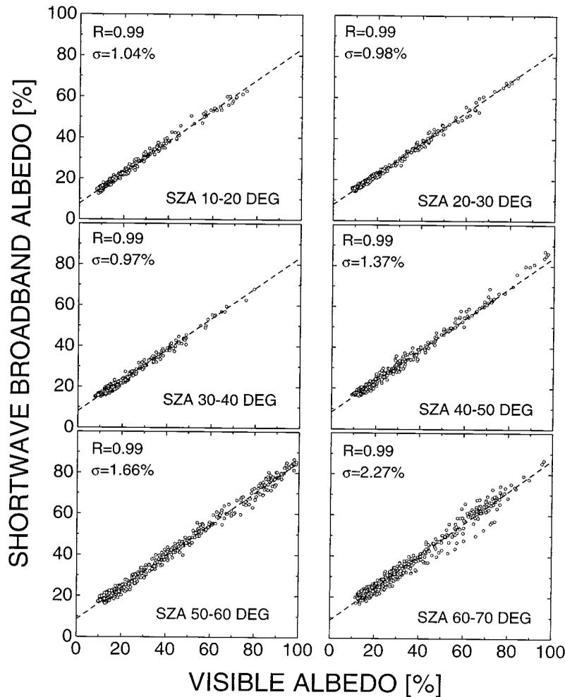
**Figure 5.** Relationship between visible and shortwave (SW) albedos observed by ScaRaB over the southern Great Plains (SGP) Atmospheric Radiation Measurement program (ARM) locale in 1994 for different ranges of solar zenith angles (SZA). Correlation coefficients  $R$  and standard deviations (SD)  $\sigma$  of the linear regressions are listed on the plots.
