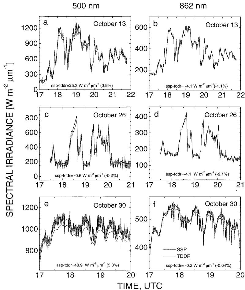
**Figure 2.** Comparison of scanning spectral polarimeter (SSP) (thick line) and TDDR (thin line) spectral irradiances at 500 and 862 nm on October 13, 26, and 30, 1995. Mean differences are listed on the plots.
