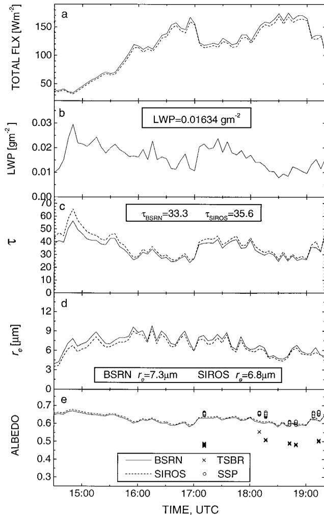
**Figure 8.** Input and output for the retrieval of cloud properties and a comparison in TOA albedo computed from ground-based measurements and from SSP. Two major input parameters are surface downwelling flux from (a) BSRN and Solar and Infrared Radiation Observation System (SIROS) and (b) cloud liquid water paths (LWP). Retrieved cloud variables are (c) cloud optical depth and (d) cloud droplet effective radius  $r_e$  from which (e) albedo were computed.
