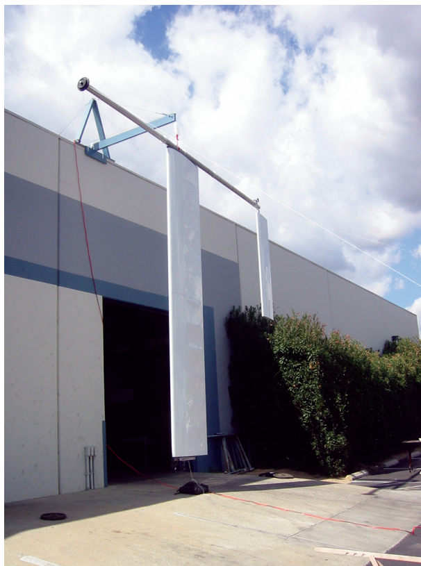
FIG. 4. A photograph of the full-scale mechanical prototype of a first-generation, single-winged balloon guidance system that was built and ground-tested under NASA funding. The main wing is 5.5 m in span with a 1.1-m chord.
