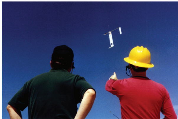
FIG. 7. A photograph from a flight test showing a 1/4-scale model suspended from a tethered blimp in windy conditions. Scale model tests were very successful in demonstrating performance and stability predictions in the Reynolds number regime in which the full-scale system will operate. A combined-system lift coefficient of 1.2 was measured at Reynolds numbers of about 45,000. For reference, the main wingspan of the model is 1.41 m, its chord is 0.308 m, and its mass is 3.4 kg.
