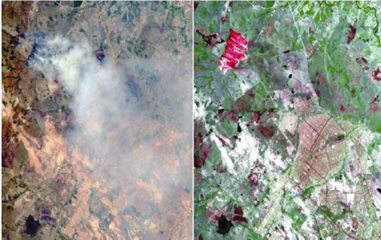
Figure 18.9 Left: a true color AVIRIS image of a fire smoke scene composited from red, green and blue channels. Right: a false color image composited from three AVIRIS SWIR channels that are equivalent to MODIS channels at 1.24, 1.64 and 2.13 \mu\text{m} (Li et al., 2004)
