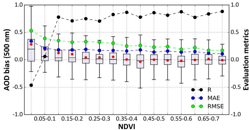
**Fig. 9.** Bias boxplots and performance of Himawari-8/AHI 500-nm AOD retrievals as a function of the normalized difference vegetation index (NDVI). The R, MAE, and RMSE in each NDVI bin is shown as black, blue, and green dots, respectively (right ordinate). (For interpretation of the references to colour in this figure legend, the reader is referred to the web version of this article.)
