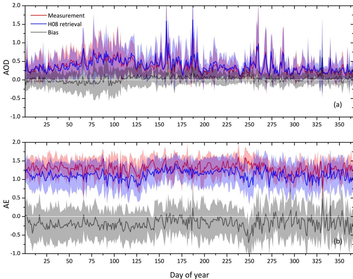
**Fig. 7.** Time series of daily-averaged Himawari-8/AHI (a) 500-nm AOD and (b) 440–675-nm AE retrievals. Ground-based measurements are shown in red. The shaded parts in each panel represent the standard deviations of the data samples. (For interpretation of the references to colour in this figure legend, the reader is referred to the web version of this article.)
