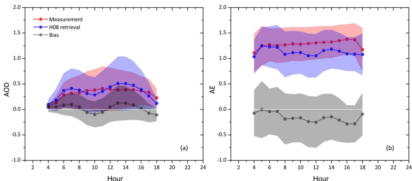
Fig. 6. Diurnal variations of Himawari-8/AHI (a) 500-nm AOD and (b) 440–675-nm AE retrievals. Ground-based measurements are shown in red. The shaded parts in each panel represent the standard deviations of the data samples. (For interpretation of the references to colour in this figure legend, the reader is referred to the web version of this article.)
