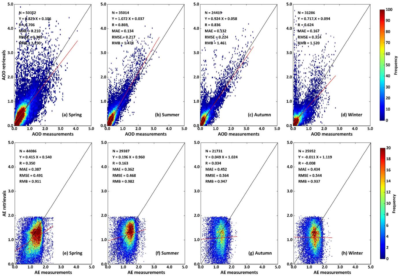
**Fig. 8.** Density scatterplots of Himawari-8/AHI (a-d) AOD and (e-h) AE retrievals against ground measurements for (left to right) spring, summer, autumn, and winter at all monitoring stations. Black lines are the 1:1 lines, and red lines are the linear best-fit lines through the data points. (For interpretation of the references to colour in this figure legend, the reader is referred to the web version of this article.)
