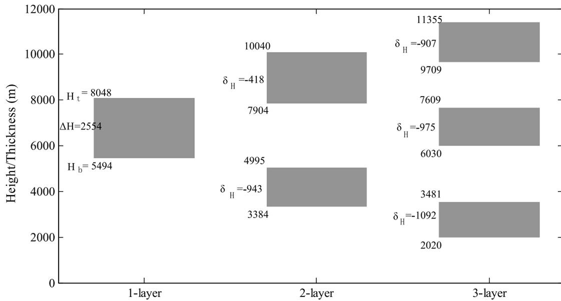
**Figure 4.** Mean locations of one-, two- and three-layer clouds.  $H_b$  and  $H_t$  are the mean cloud base height and cloud top height for each cloud type, respectively.  $\Delta H$  is the mean thickness of one-layer clouds;  $\delta_H$  is the difference in thickness between each layer of cloud in a multilayer cloud configuration and one-layer clouds. Units are in meters.
